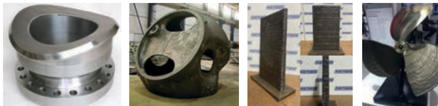
Examples of WAAM: (a) a stainless steel self-reinforced flange (Gainza forge, Spain); (b) a cast wind turbine rotor hub; (c) a large steel plate made by WAAM; (d) a blade made by WAAM.
