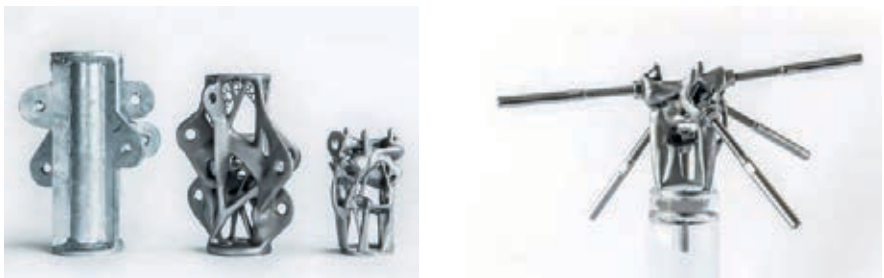
Design evolution of a typical node in tents as in Pompidou-Metz Centre submitted to six different inclined tension forces – From traditional welding to additive manufacturing – Final node with tension rods in place – Credit to Salome Galjaard @ Arup
