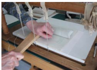
Sewing the textblock: controlling swell with a consolidation stick (left) and the finished sewing (right).
