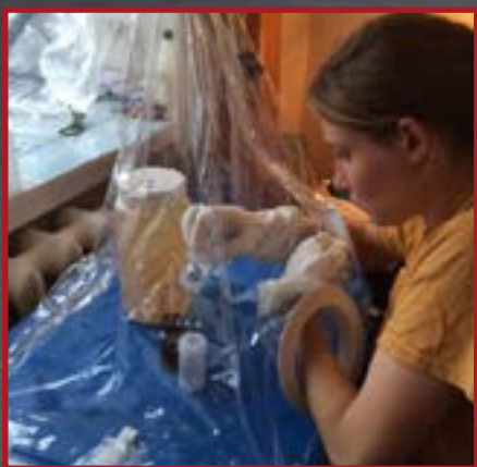
Cat separating colloids and particles in a portable field "clean-room" to prevent contamination.
